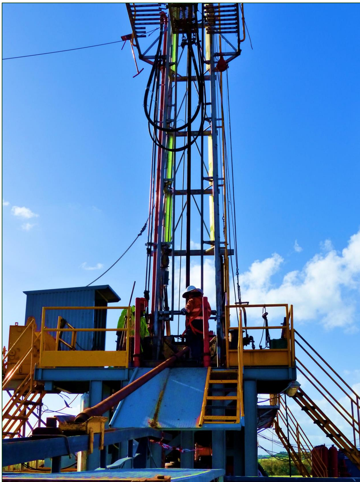
DCA personnel making a connection as they drill an 8 ½" hole toward the primary objective.
