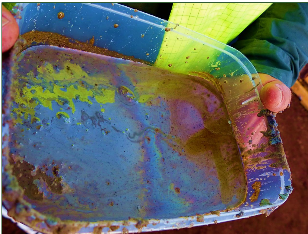
Sand from the Bookara Sandstone being examined by the Wellsite Geologist (top) and a sample of the oil film collected from the ditch cuttings from the top section of the Bookara Sandstone (below).
