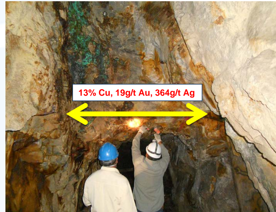
Selective underground mining of high grade copper veins at Promontorio
