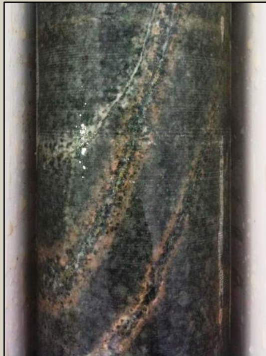
Figure 10 – K-spar selvages (pink) to quartz-chalcopyrite 'B' veins (HQ diameter drill core).
