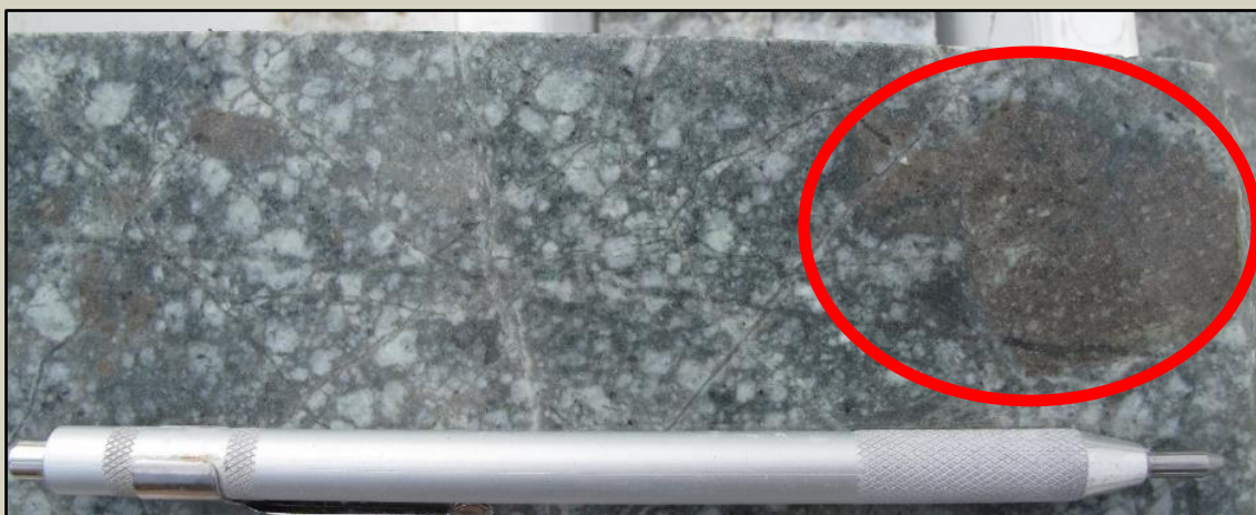
Figure 5 – Biotite altered xenolith at 293m depth.
