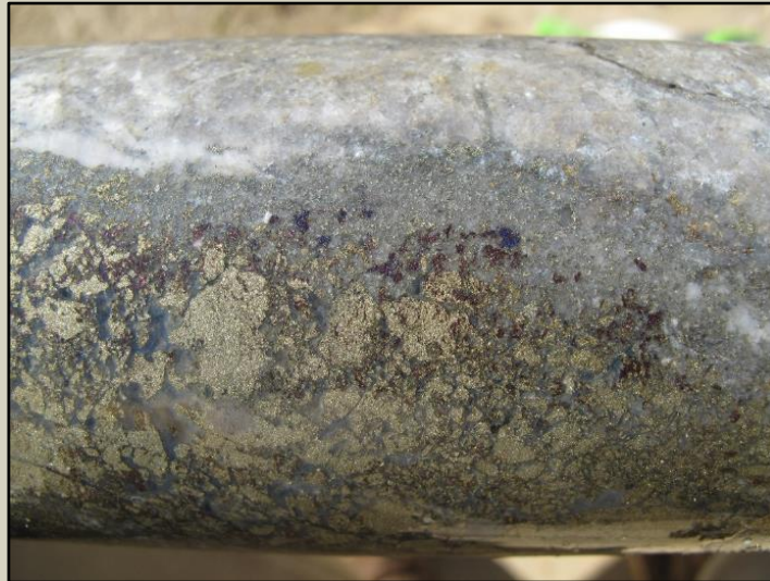
Figure 8 – Bornite in a quartz-pyrite-bornite-chalcopyrite sulphidic vein at 340.6m (bornite is the purple sulphide – hence its colloquial name ‘peacock ore’).
