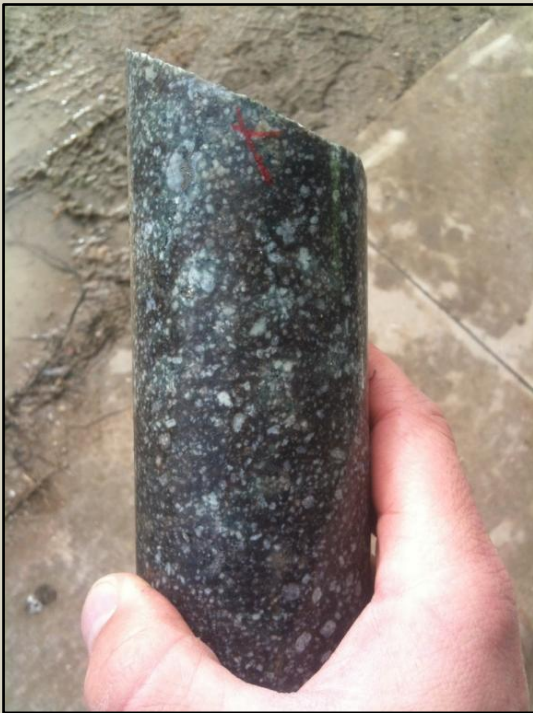
Figure 9 – Pervasive biotite (potassic) alteration (dark brown groundmass).
