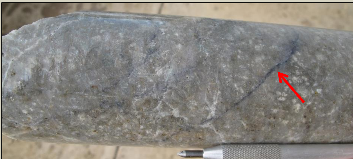
Figure 7 – Silica-sericite altered rock with fine molybdenite veining at 261.5m.
