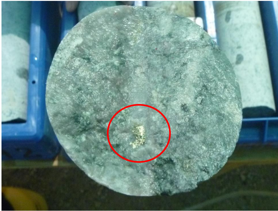
Figure 4 - (drillhole depth 238.0 m) Disseminated chalcopyrite in quartz-pyrite veinlets (1cm wide) dioritic intrusive, moderate potassic alteration (secondary biotite, magnetite, orthoclase) with moderate silicification.
