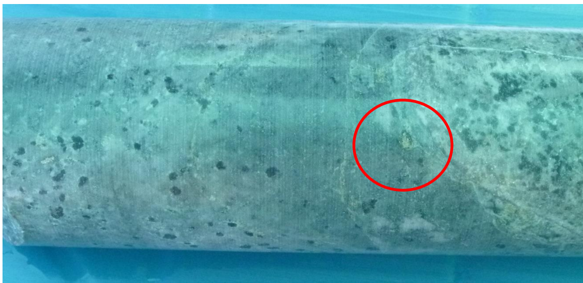
Figure 6 - (drillhole depth 273.65m) Chalcopyrite in epidote-quartz veinlets (0.1cm wide), diorite intrusive, moderate potassic alteration (secondary biotite-orthoclase), moderate silicification.
