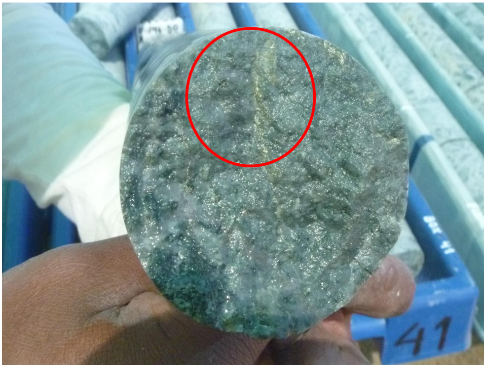
Figure 5 - (drillhole depth 269.5m) Chalcopyrite in quartz-epidote-pyrite veinlet (0.1cm wide) hosted by diorite intrusive with moderate potassic alteration (secondary biotite-chlorite-orthoclase) and moderate silicification.
