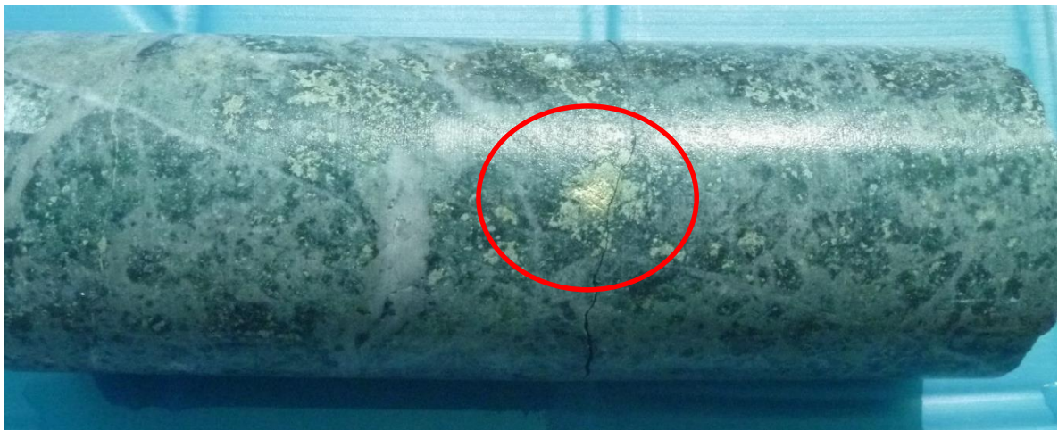
Figure 2 - (drillhole depth 188.70 m) Chalcopyrite disseminated in volcanic andesitic crystal tuffs, strong potassic alteration (secondary biotite, orthoclase) with pyrite-quartz stockwork. veinlets
