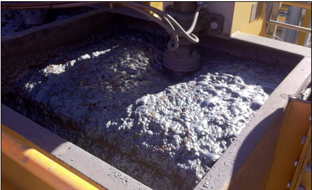
Lead-zinc concentrates being produced in the cleaner flotation cells.
