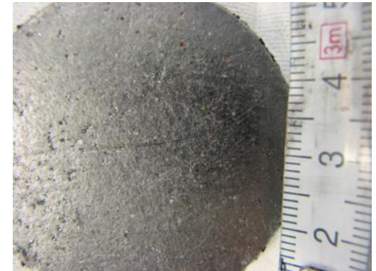
Graphite foil produced from Kibaran large flake graphite
