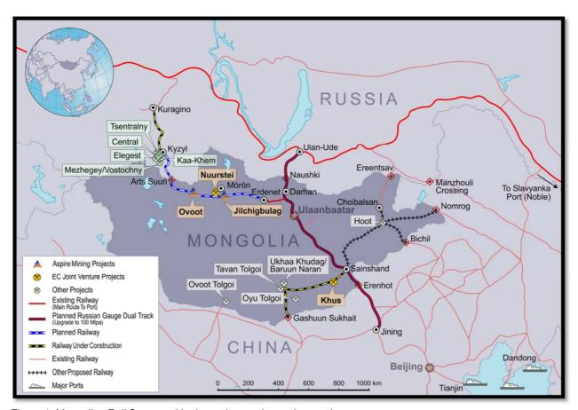
Figure 1: Mongolian Rail System with planned upgrades and extensions
