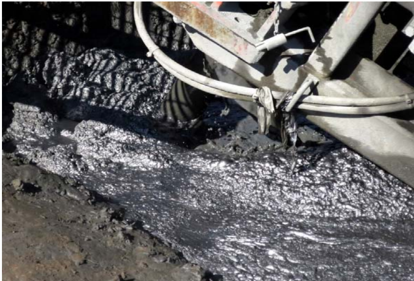
Graphite liberation as seen at surface on diamond drill hole GBND0005
