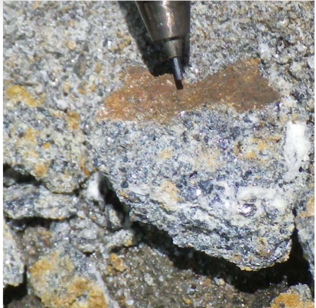
Close up image of the graphite-bearing quartzose schist found on exploration license 5304
