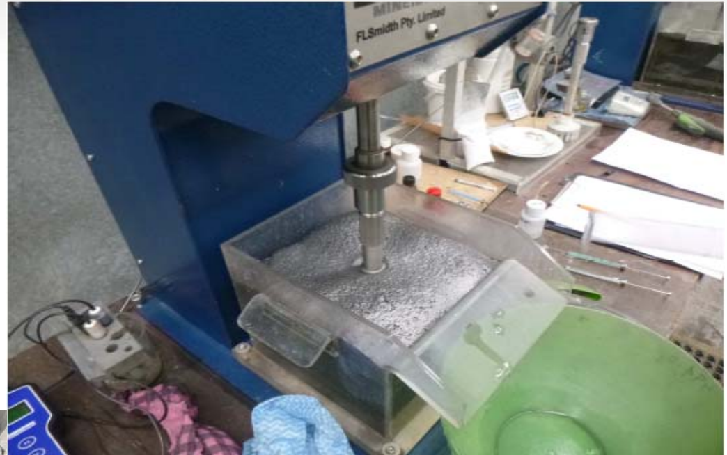
Image of the graphitic material being liberated using a flotation method at the ALS Metallurgy laboratory
