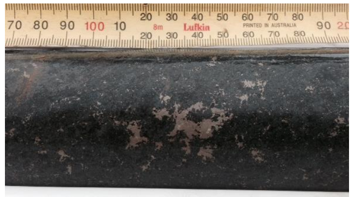
Figure 2: Blebby pyrrhotite and chalcopyrite of probable magmatic origin. HQ drill core from RBDD004, 96m depth.
