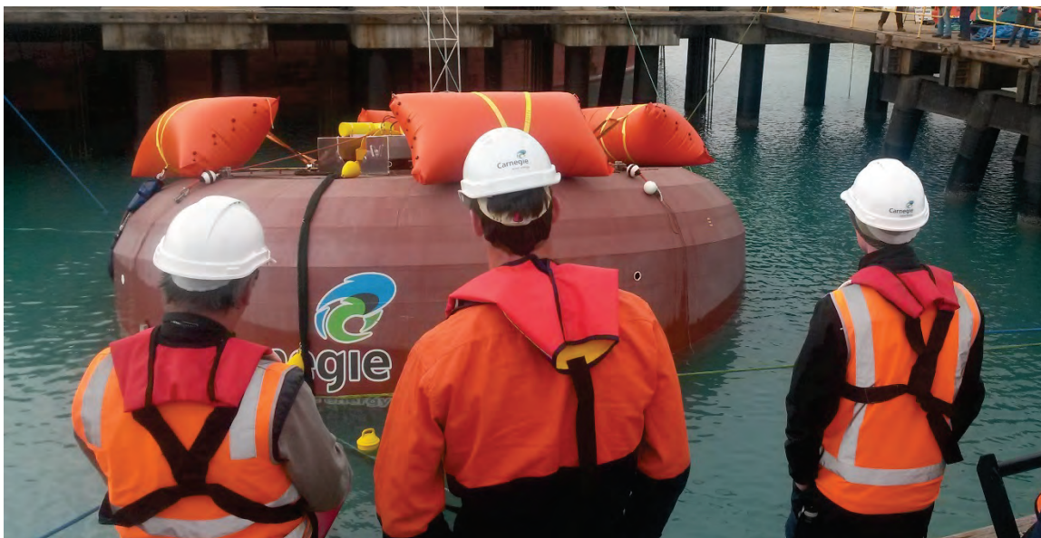
In-ocean testing of the CETO 5 Unit 1 Buoyant Actuator
