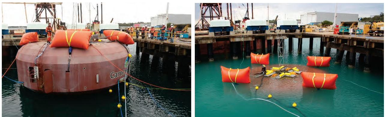
In-ocean testing of the CETO Unit 1 Buoyant Actuator
