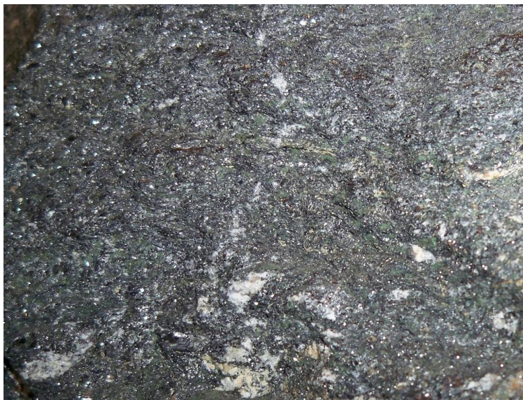
18 Graphitic gneiss containing 16.5% TGC + 0.3% Vanadium
