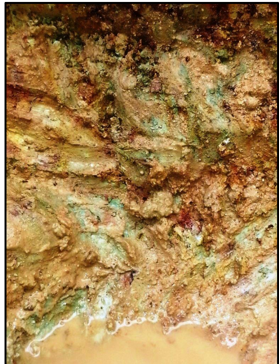
Figure 7. Intersection of a highly micaceous dyke in LPTR 003 (Eastern bore-hole cluster). A second, less micaceous feature has also been intersected, with a coarser mineralogy showing up in pan concentrates.
