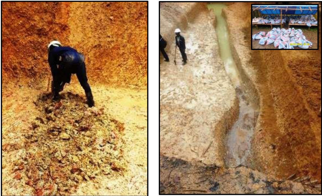
Figure 6. Photographs showing collection of kimberlite dyke material by hand, for eventual processing through the 40 tph head feed DMS plant.
