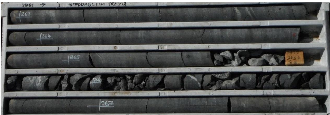
Figure 2: Core tray #18 from 14MPDDHBGC1W1 from 262.95 to 267.65m, showing typical dark grey graphitic core.
