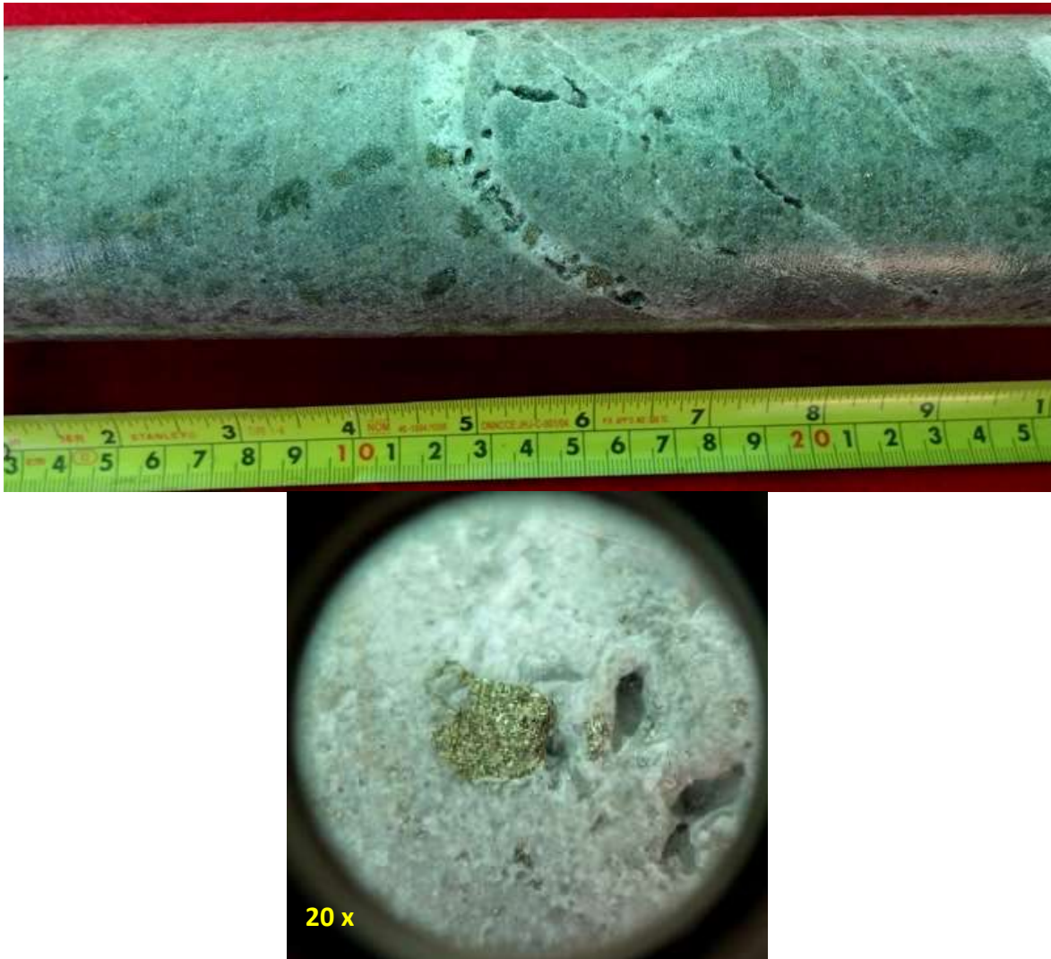
Figure 2 – (Drill Depth 283.35m) Quartz-pyrite-chalcopyrite-sericite veinlet. 6mm wide in strongly pyritic altered andesite tuff with disseminated pyrite.
