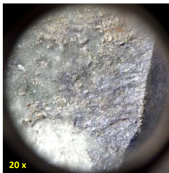
Figure 4 – (Drill Depth 430.10m) Quartz-molybdenite-calcite veinlet, 2mm wide in andesitic tuff with strong phyllic alteration and 2% disseminated pyrite.
