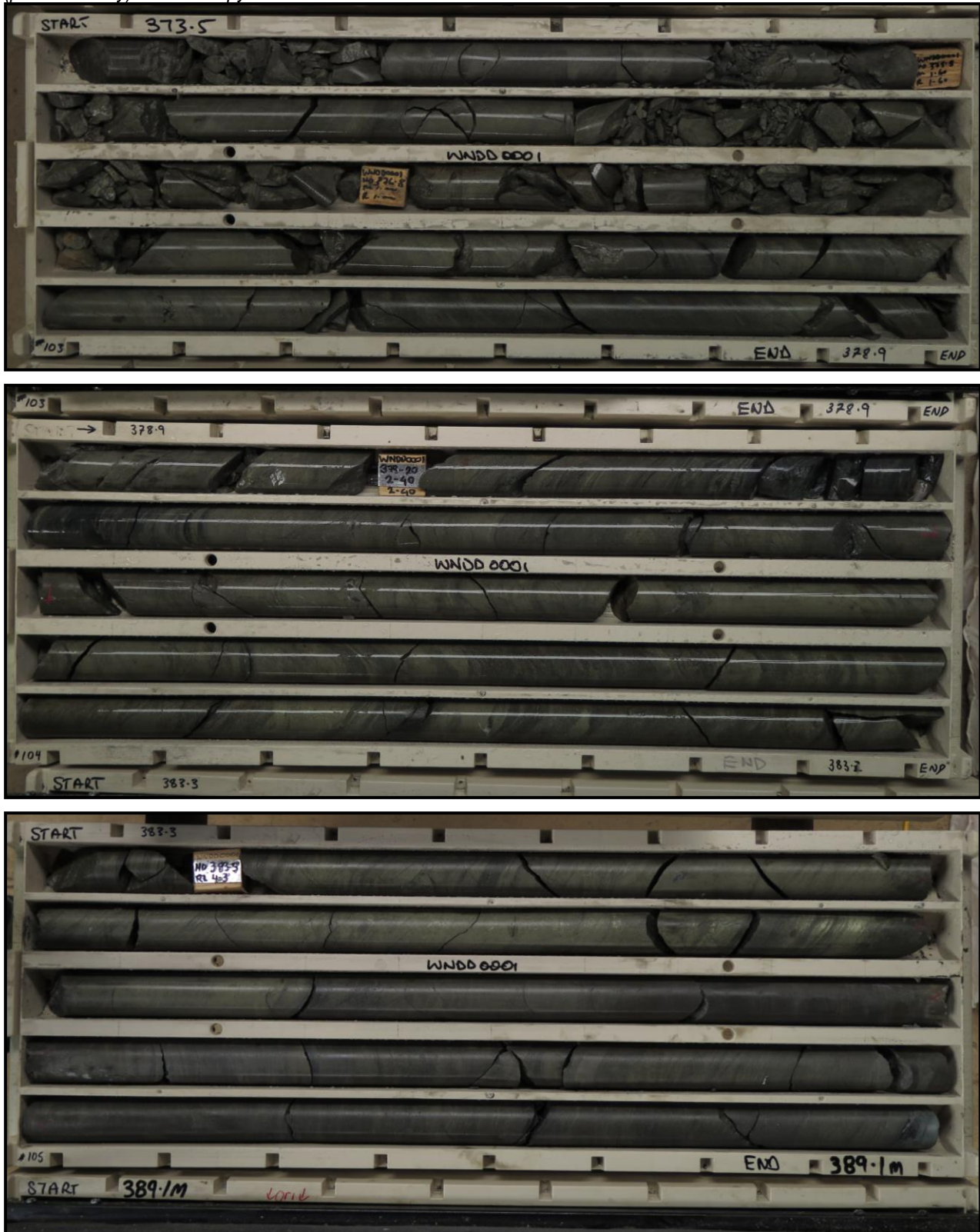
Figure 1: Drill core photographs from WNDD0001 showing mineralised intercepts from 373.6m to 389.1m. The fine-grained black minerals are predominantly galena and sphalerite, whereas the yellow minerals are a mixture of pyrite (predominantly) and chalcopyrite.
