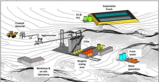
Etango Heap Leach Cribs - four 2m x 2m x 6m columns
