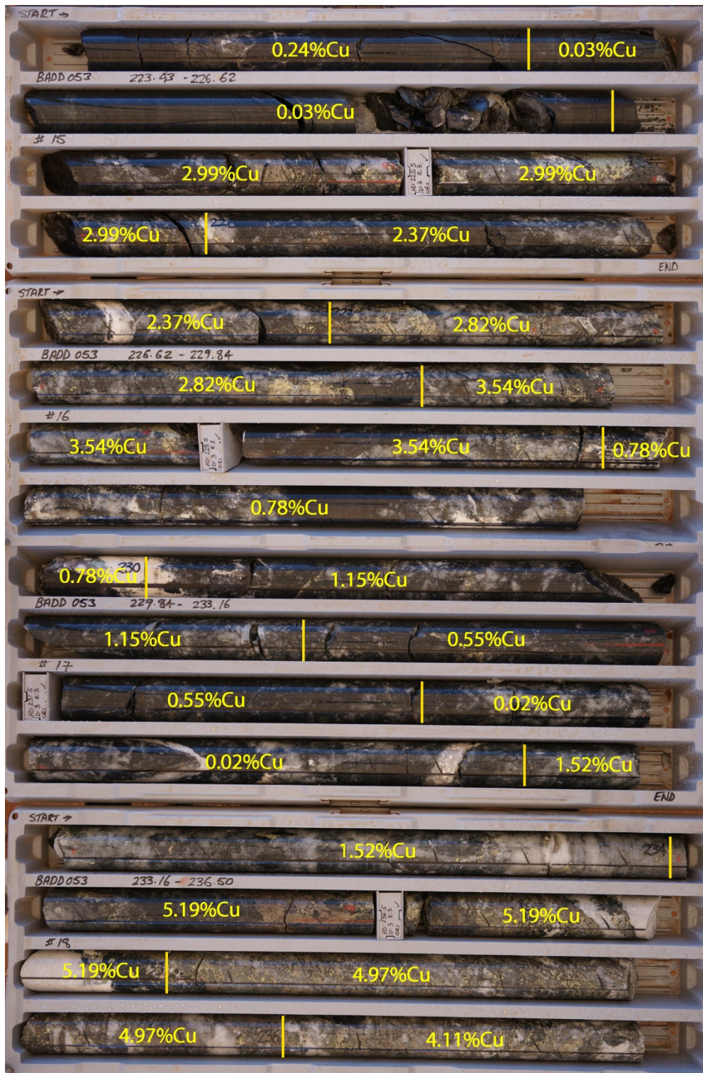
Figure 3 - High grade copper (coarse grained chalcopyrite) mineralisation in BADD053. Mineralisation associated with sheared quartz – carbonate veining and biotite schist in the Hangingwall Lode position is illustrated. Chalcopyrite mineralisation development from 225 to 257.5 metres downhole. True width is approximately 85% of downhole width.
