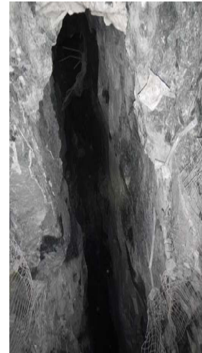
Photo : Shows example of a narrow vein bench stope
