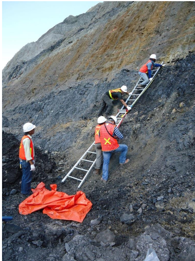
Figure 2: Sampling coal seam on TCM highwall
