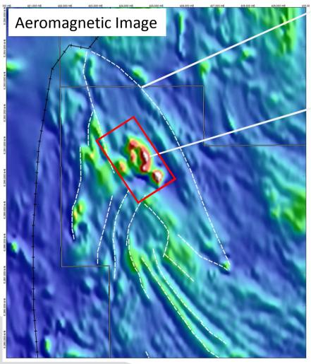
Aeromagnetic Imagery shows an 8 kilometre long, NW-trending oval structure
