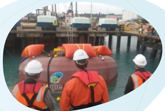
CWE personnel overseeing Buoyant Actuator in-ocean testing
