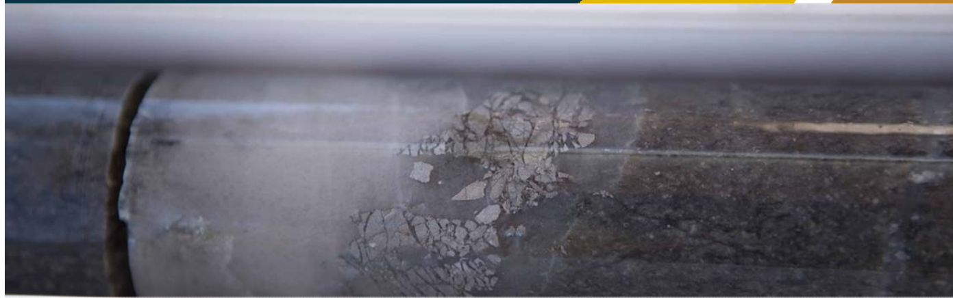
Gruyere drill core, 14GYDD0008 – Arsenopyrite vein
