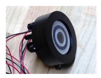
Figure 1 – Miniaturised prototype unit (55mm diameter, 20mm tall, 87 grams weight)
