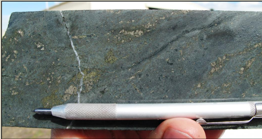
Figure 14 – Patchy to disseminated pyrite and chalcopyrite sulphide mineralisation associated with biotite and potassium feldspar (potassic) alteration in SMD002 – 335m.
