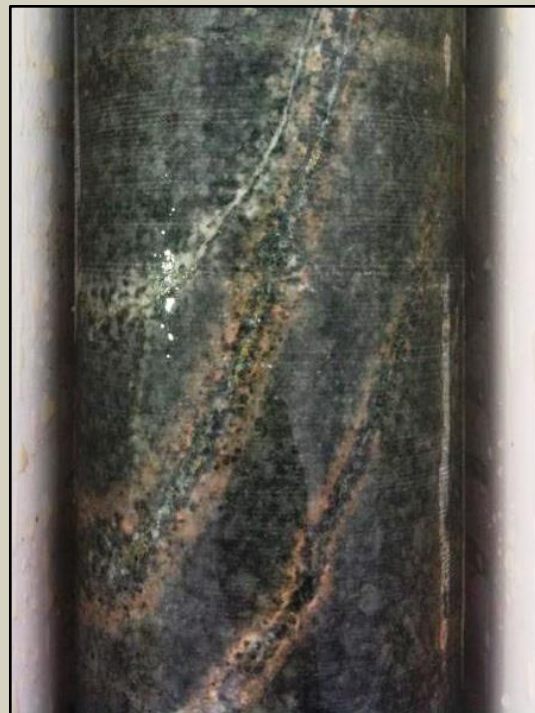
Figure 12 - K-spar selvages (pink) to quartz-chalcopyrite 'B' veins (HQ diameter drill core).
