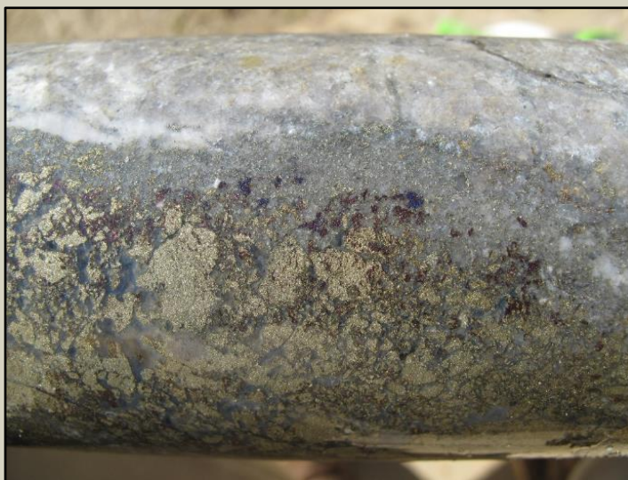
Figure 2 - Bornite in a quartz-pyrite-bornite-chalcopyrite sulphidic 'D' vein at 340.6m (bornite is the purple sulphide – hence its colloquial name 'peacock ore').
