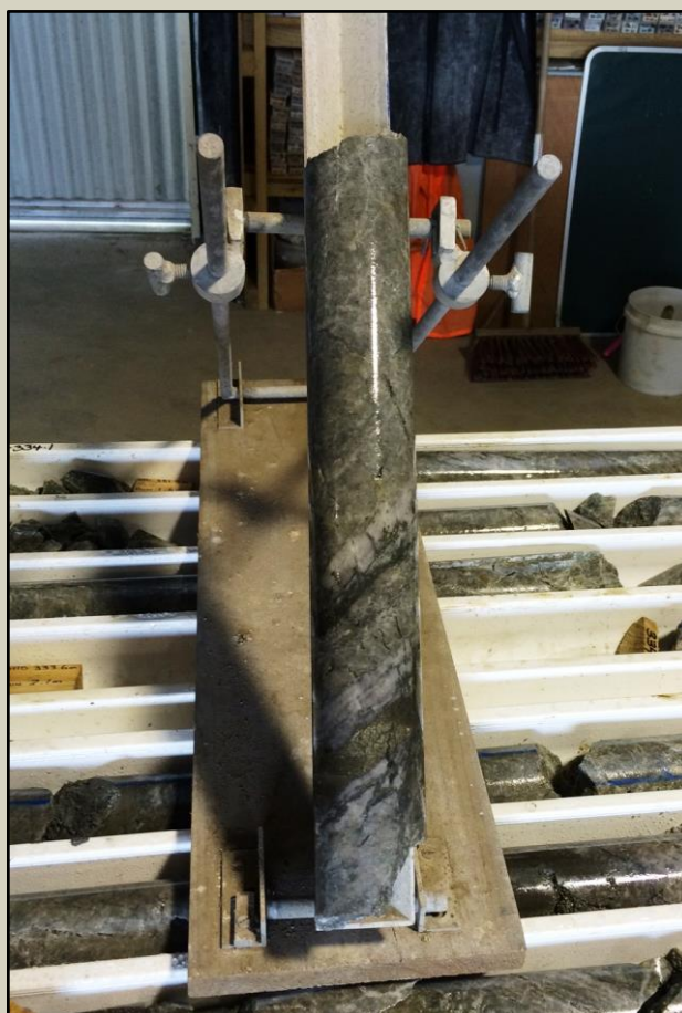
Figure 3 - Oriented 'D' vein at 340m depth in SMD003 demonstrating a 55 degree dip towards the south (to the left of picture).
