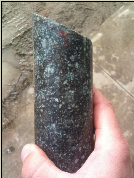
Figure 11 - Pervasive biotite (potassic) alteration (dark brown groundmass).
