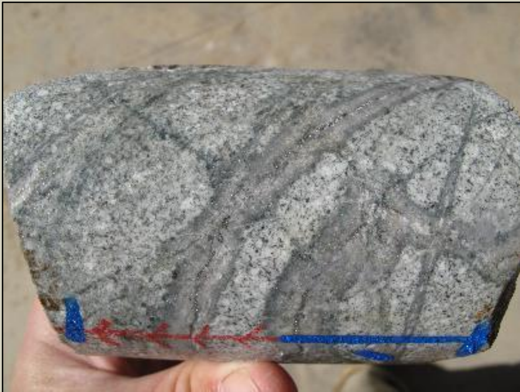
Figure 6 - ?Tonalite with stockwork quartz pyrite veining at 182m.
