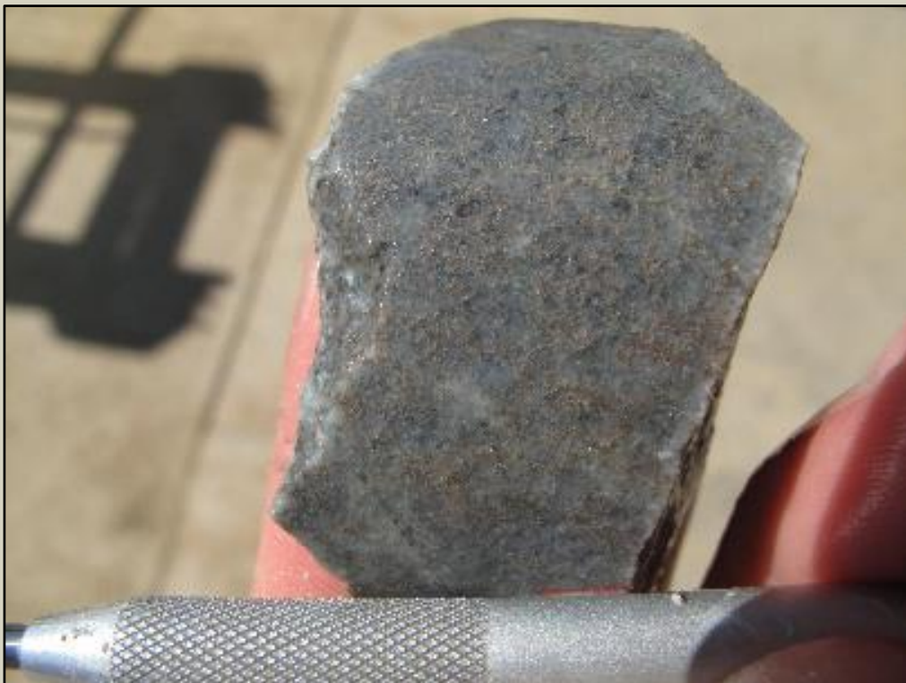
Figure 7 - Brown hydrothermal biotite at 369m.
