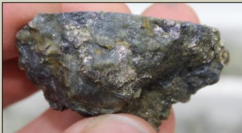
Figure 10 - Bornite in 'D' vein at 402.3m.
