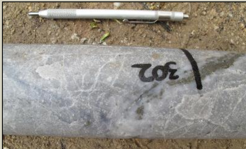
Figure 8 - Silica flooded zone at 302m with silica-pyrite-?ankerite alteration and quartz-pyrite-molybdenite veining. Similar to zones in SMD003 at 263m and 340m.
