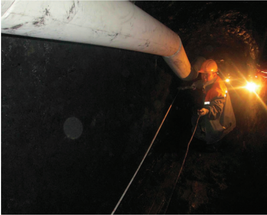
Photo 2: Showing a miner working within the bulk sample decline shaft with lighting and air ventilation.
