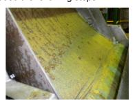
Rougher and Cleaner Spirals delivered improved recoveries to Heavy Mineral Concentrate when trialled with pre-screened ore.
