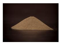
Gravity and conductivity separation were confirmed to be an effective means of separation and recovery of T65 product (leucoxene).
