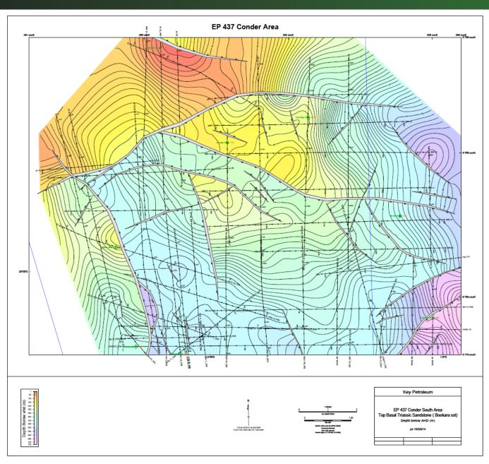
The Conder Area in the northern part of EP437 has several structural highs (yellow and orange) that the Operator is currently mapping as follow up drilling prospects in conjunction with other mapped prospects in the area. The central high (middle of diagram) is undrilled and on trend with the Dunnart structure, intepreted to be on the main oil migration pathway.
