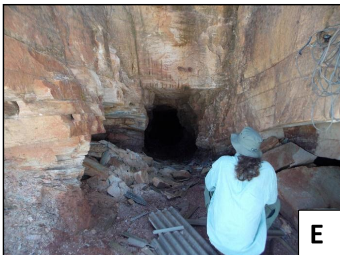
Photos- (A) Garimpo; (B) Garimpo with Faina at the background; (C) Garimpo: power generator; (D) One of the several winze entrances; (E) Winze portal following the mineralised quartz vein; (F) Detail of the mineralised quartz vein and biotite alteration halo.
