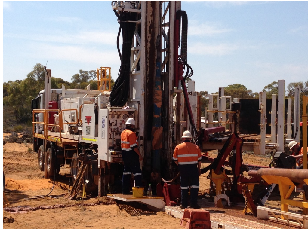
Metallurgical bulk sample drilling using 8" diamond core
