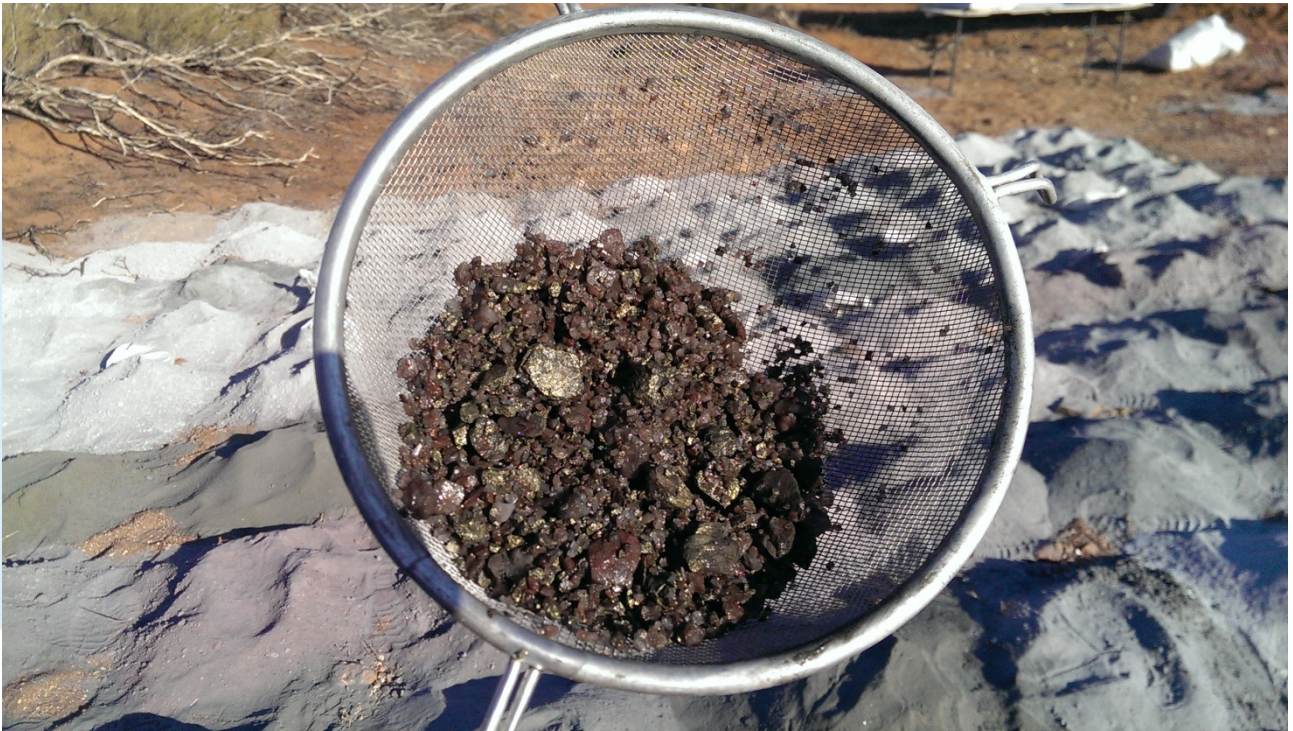
Figure 2: RC chips of massive copper sulphide mineralisation from hole BYRC009
