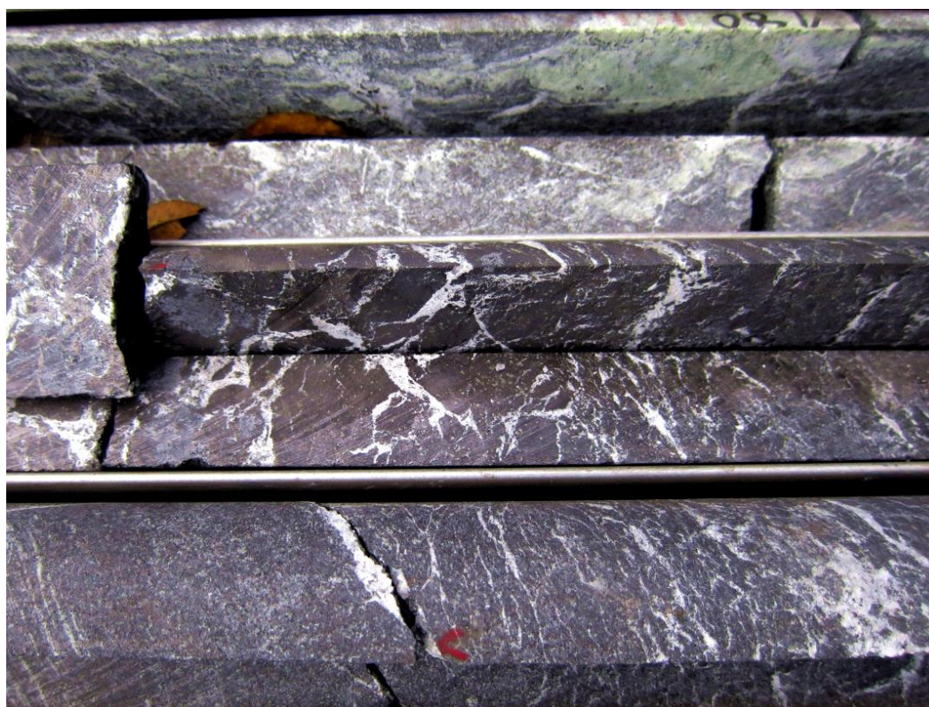
Figure 1. Diamond drill core from Nicanda Hill showing a possible hydrothermal breccia zone.
