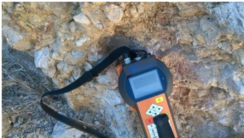
Figure 5: Mineralized Breccia with 11796 CPS and disseminated pyrite+sulphides.
