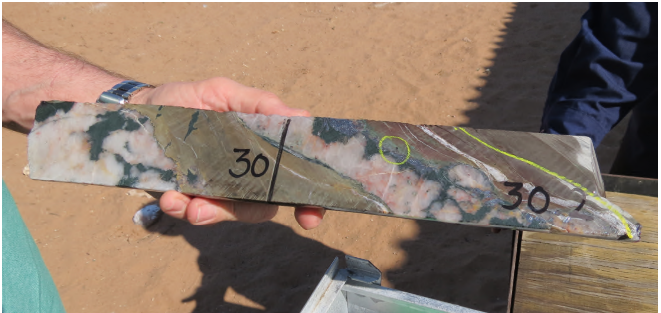
Figure 1: Chalcocite mineralisation (grey) along margins of veins at 30m depth in drill hole MO-116-D
