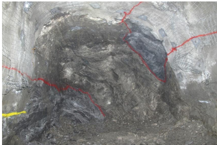
255 North ore drive face with 7% nickel massive ore
