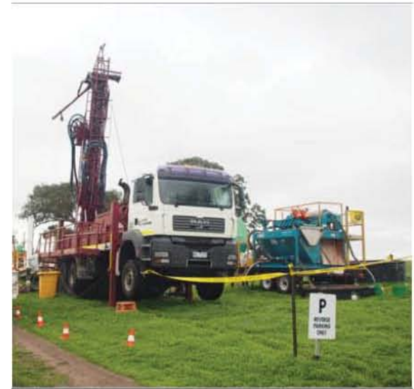
No sumps – closed loop system
