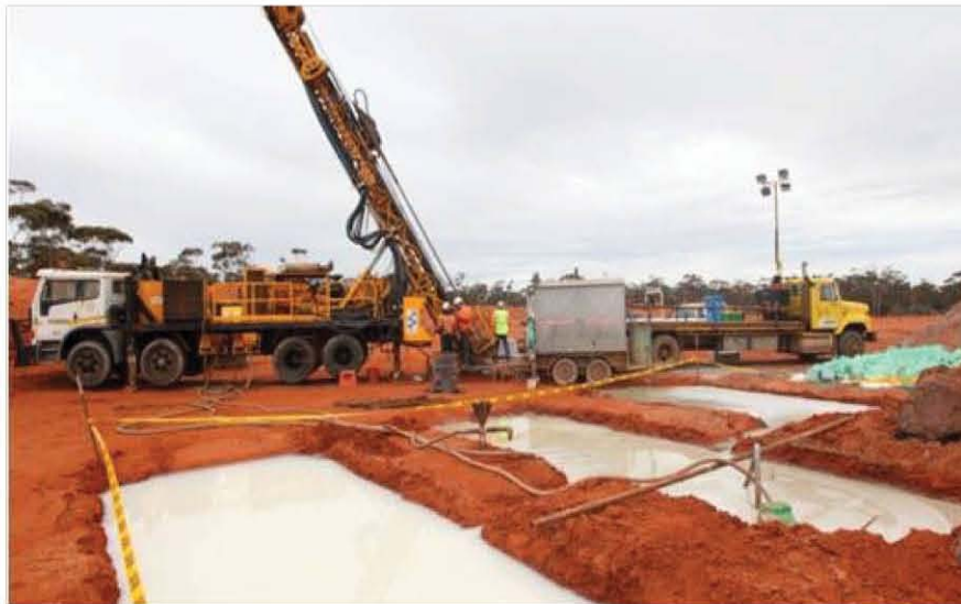
Traditional drilling fluid sumps
