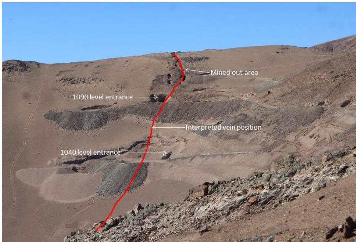
Figure 2 – San Sebastian mine and vein looking north. Note favourable topography for access, vertical distance between the 1040 level and 1090 level entrances is approximately 50m. Work is planned to establish additional mining access tunnels into the vein below the 1040 level.
