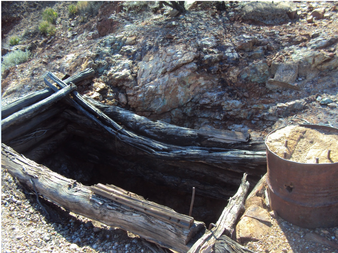
Figure 4: Old Prospecting shaft at Bonya Mine, also showing outcropping oxide copper mineralisation (green staining on rock outcrop behind shaft collar)
