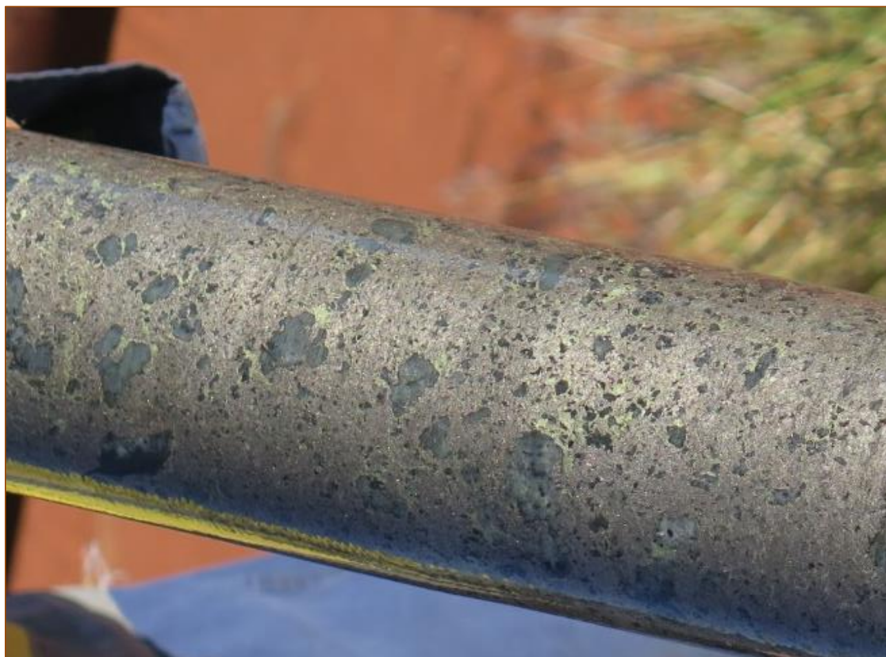
Figure 3. Coarse pentlandite and chalcopyrite mineralisation with pyrrhotite.
