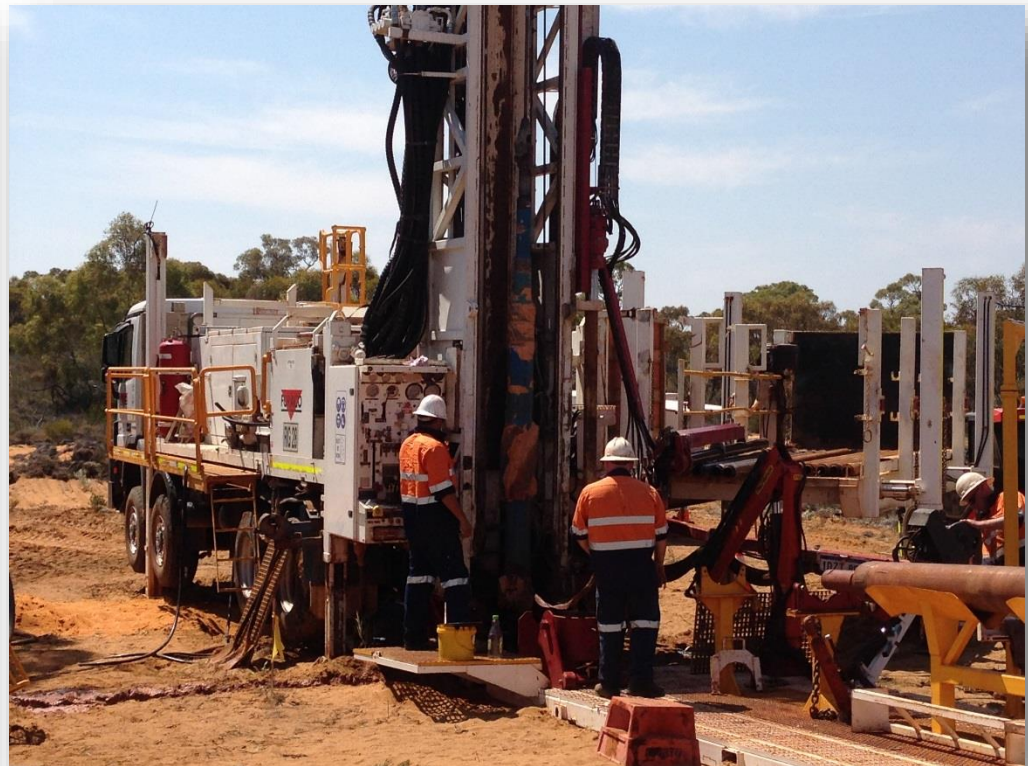
Metallurgical bulk sample drilling using 8" diamond core
