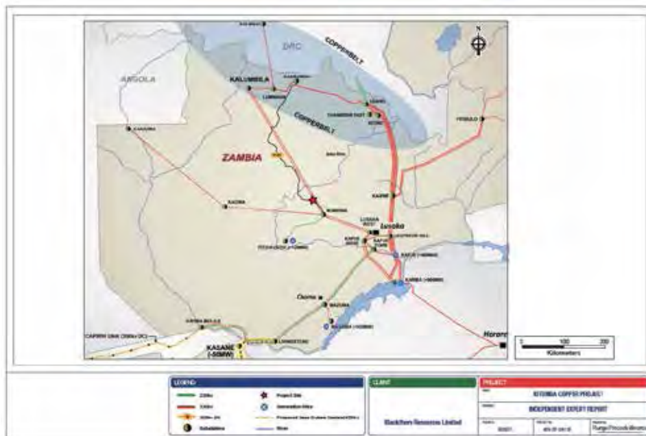
Figure 10.1 – ZESCO Current and Proposed Electricity Distribution Grid
