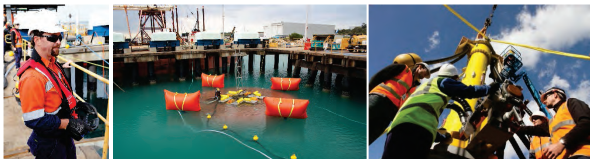
Carnegie employee (left) controlling in-ocean testing of the Buoyant Actuator (centre), onshore pump integration testing (right)
