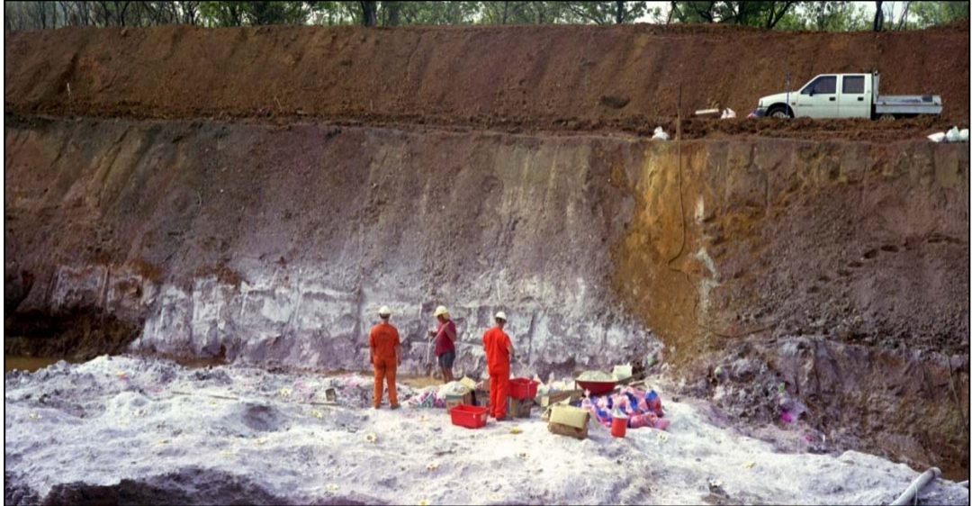
Figure 3 Test mining of magnesite at Winchester deposit. Crew standing on top of the magnesite mineralisation which extends at least several hundred meters laterally and to at least 100m depth.
