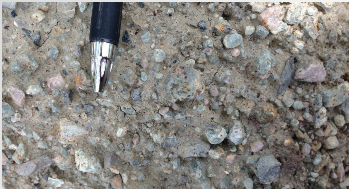
Figure 4. Variably silicified and pyrite altered sediments at Lingokoto Project
