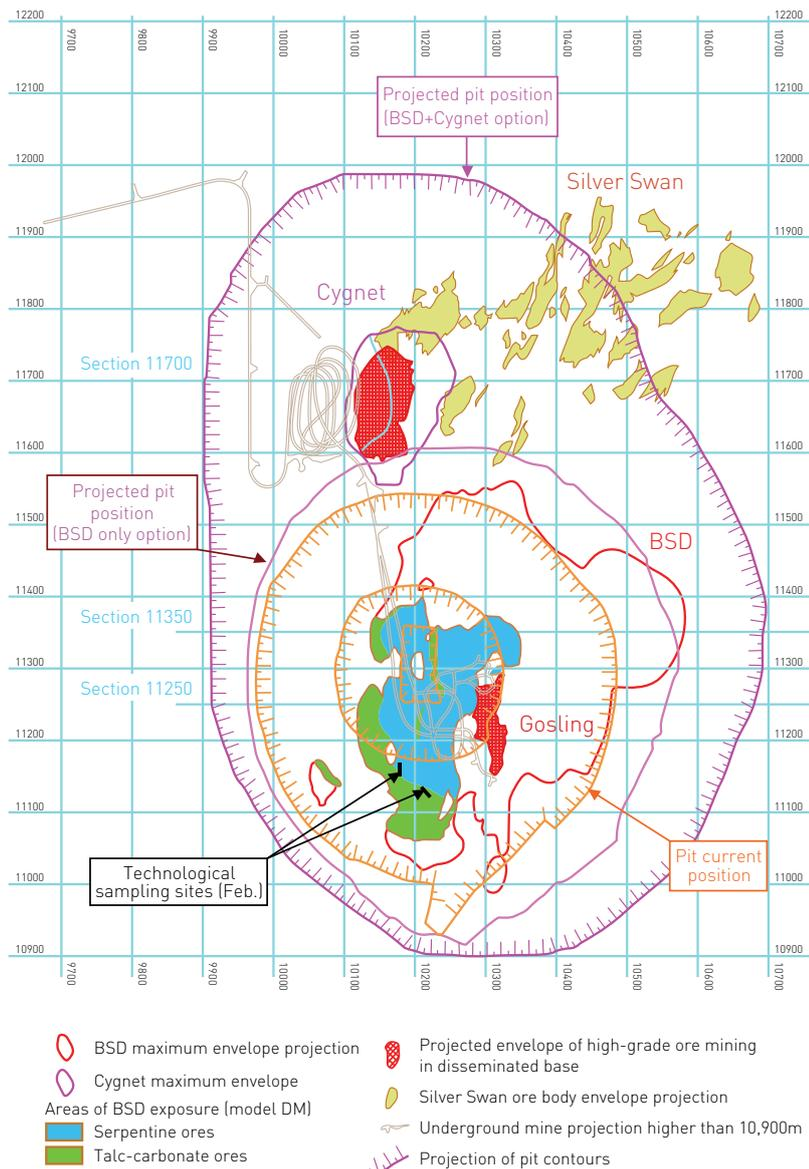
Figure 4: Black Swan Disseminated (BSD) and Cygnet mineralisation with existing mining infrastructure and pit shell options
