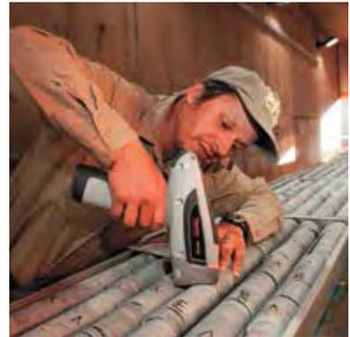
Innovation has saved us time and money. This portable XRF analyser is able to give us critical insights into rock mineralogy in real time rather than in weeks previously. We can now constantly adjust our drilling programmes using fast feedback even as a hole is being drilled.
