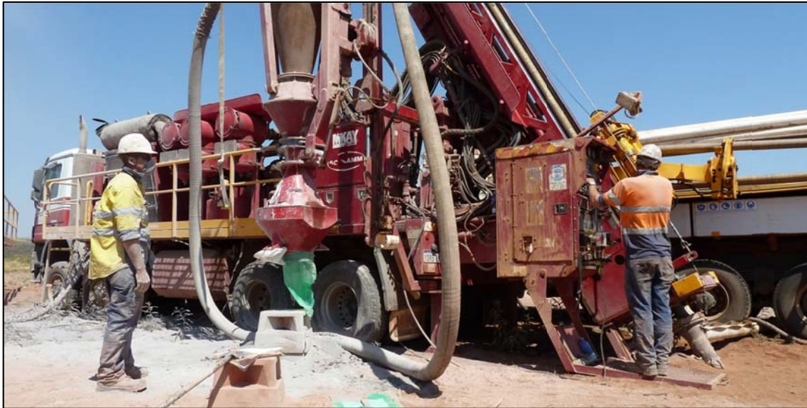
Figure 1 – Phase II RC drilling operations, Bluebird Prospect, Tennant Creek
