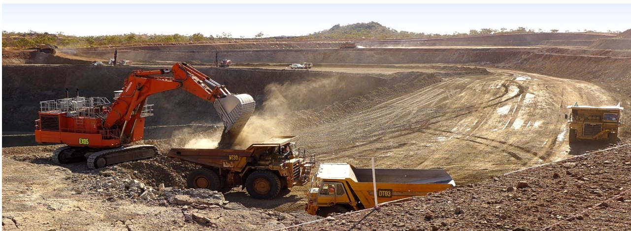
Figure 48: Mining waste from the north-east shoulder of LM2 whilst with blast-hole drilling takes place on the north-west shoulder of LM2 in the background.
