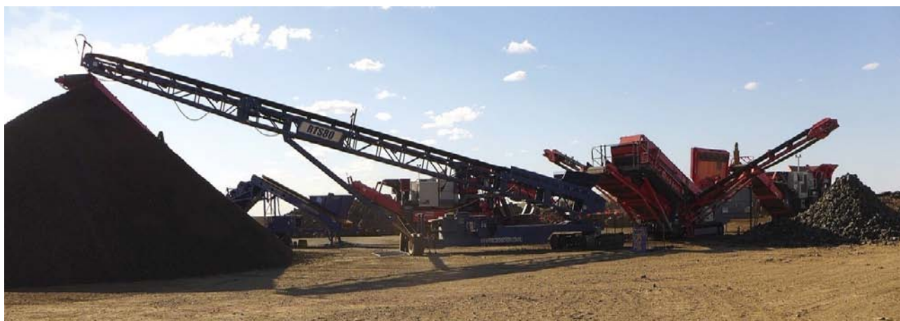
Figure 53: Mobile crusher configuration with +40mm crushed product on left, +110mm scalped product on right and -40mm product obscured behind crusher (bottom image).
