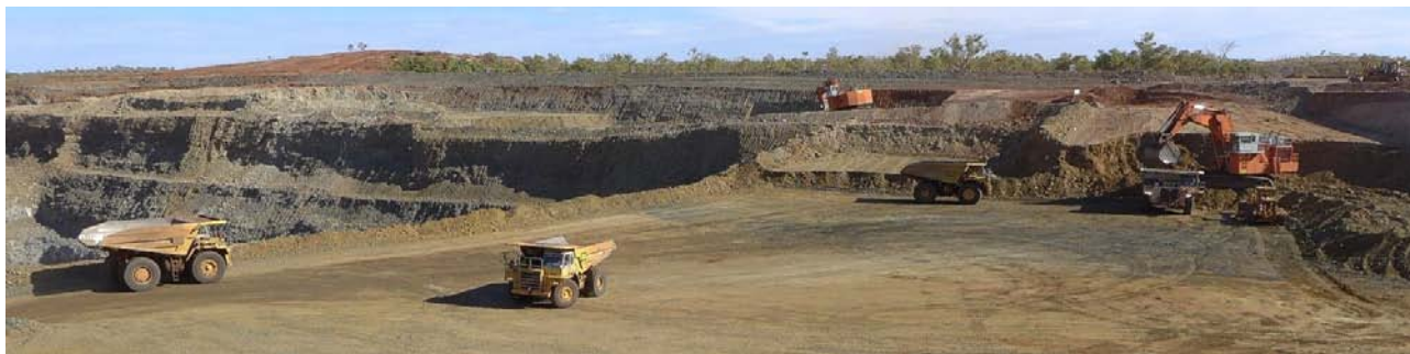
Figure 49: Mining ore and waste on the north-west shoulder of LM2 pit after blasting.
