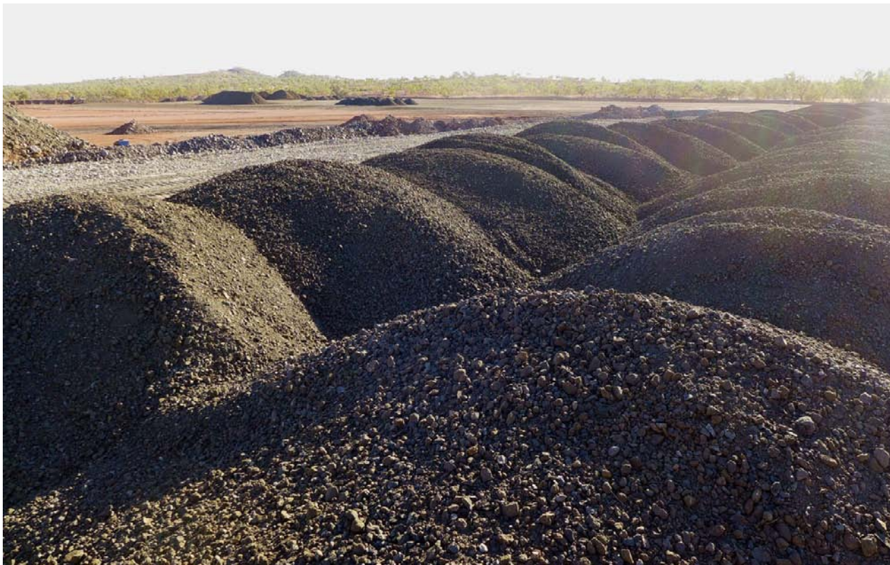
Figure 12: Crushed native copper ore stockpiles - ready for upgrading through the Company's new ore sorter, which was under construction in Hamburg Germany during the Quarter.
