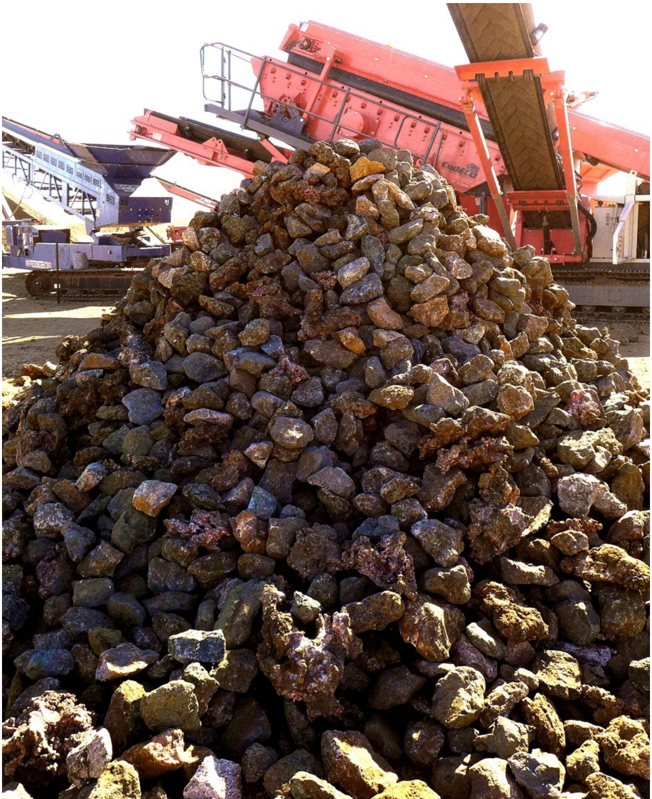
Figure 17: Scalped coarse DSO (+110mm) product includes coarse native copper nuggets, coarse and fine native copper in rock matrix (native copper contains 99.65% Cu), chalcocite masses, blebs and infill (79.9% Cu), cuprite (88.8% Cu) and various secondary copper species, visually estimated at ~30% Cu in this batch.
