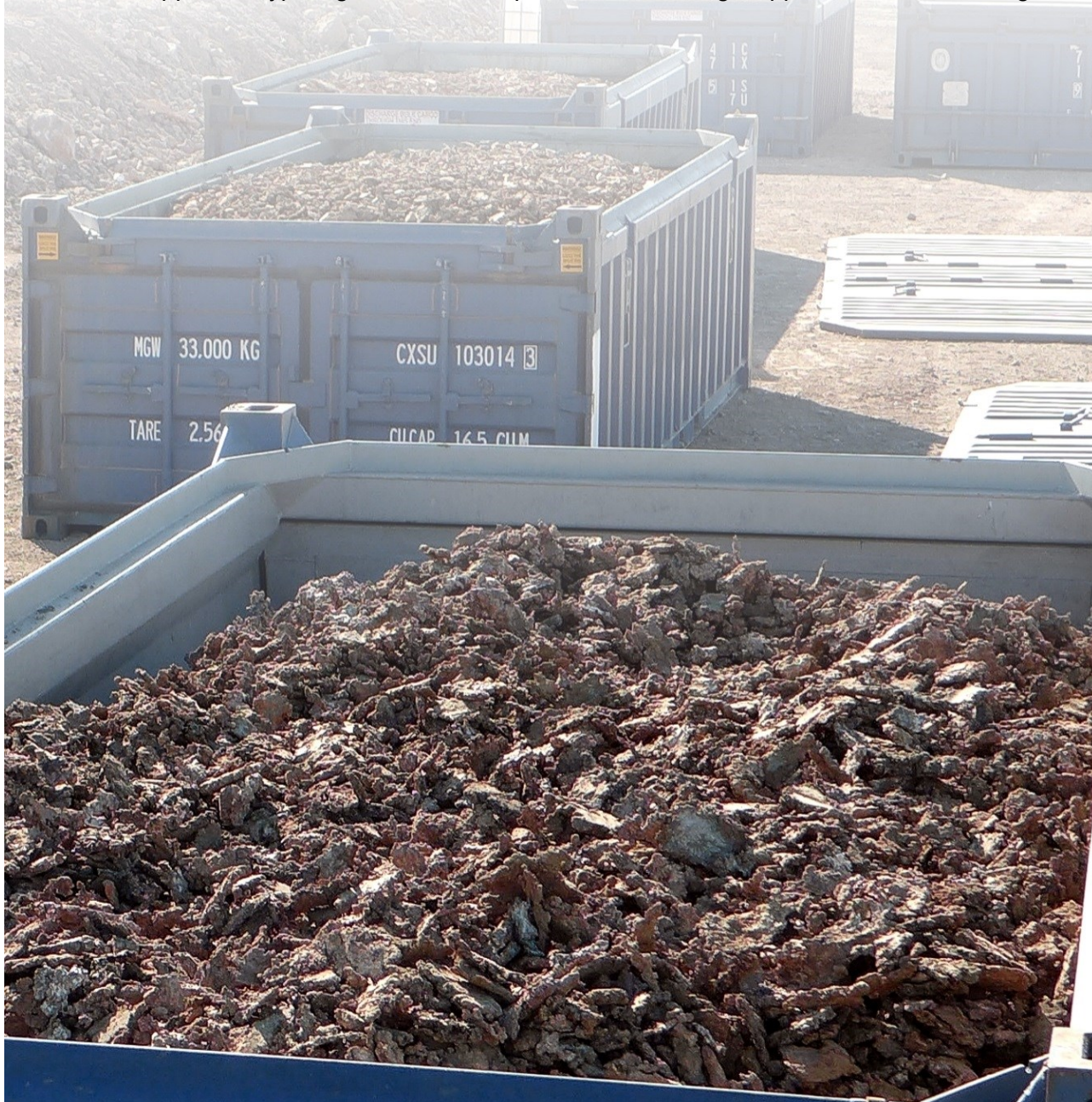
Figure 14: High-grade DSO (+40mm) visually estimated at 80-90% Cu, scalped off the crusher screens and loaded into containers ready for shipment. Each container holds between 22-25 tonnes of predominately native copper (99.65% Cu), with cuprite (88.8% Cu), chalcocite (79.9% Cu) and various supergene copper species.
