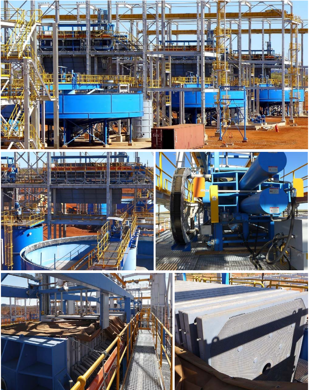
Figure 29: Thickener/Filtration circuits (above) and close up of filtration unit and panels (bottom images)
