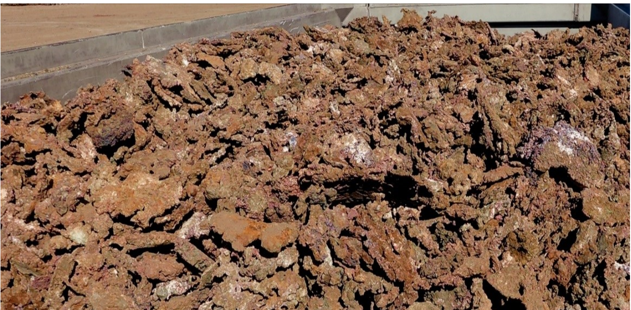
Figure 7: Container full of DSO straight from the crusher screens estimated 85-95% Cu, (+40mm -110mm)
