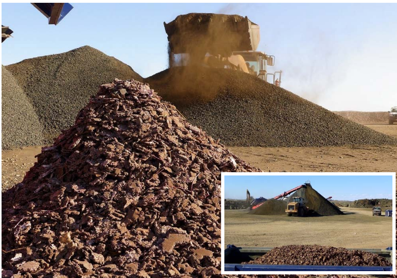
Figure 15: High-grade DSO (+40mm) scalped off the crusher screens. Predominately native copper (99.65% Cu), with minor cuprite (88.8% Cu) and chalcocite (79.9% Cu) and various supergene copper species. Inset; crushed product under the -40mm conveyors and +40mm scalped native copper DSO product in containers in foreground.
