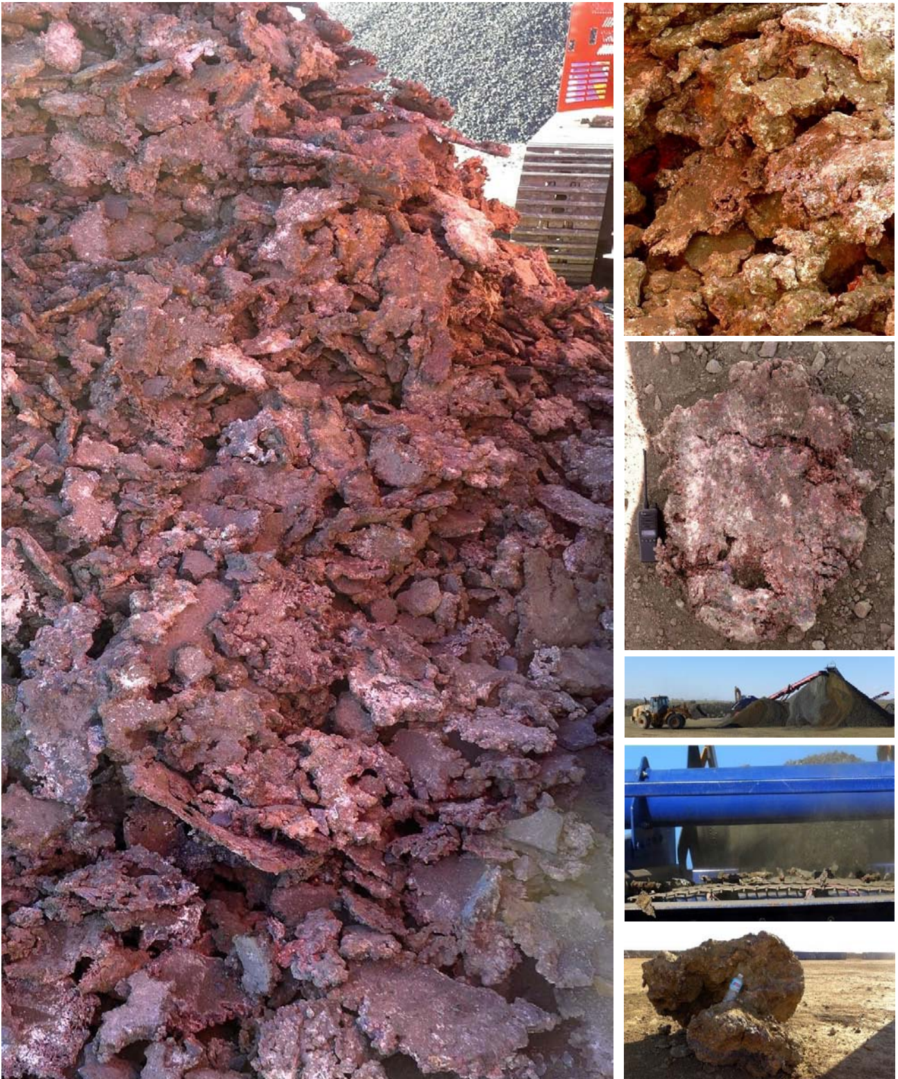
Figure 18: Left; high-grade DSO (+40mm) visually estimated at 90% Cu in this batch, scalped off the crusher screens - predominately native copper (99.65% Cu). Right (top to bottom); close-up of +40mm scalped product; large 60kg copper nugget; -40mm crushed product; containers of +40mm scalped product; up-close detailed image of operating +40mm screens showing flattened native copper being removed; and large native copper nuggets of predominately native copper on the ROM with DSO containers in the background.
