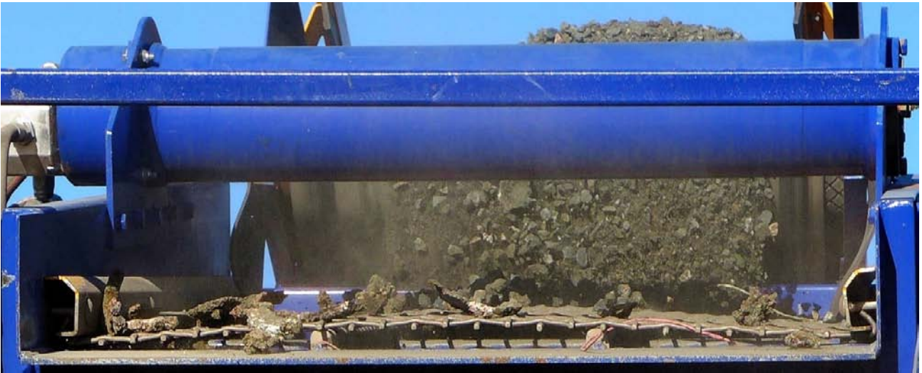
Figure 54: At the mobile crushing circuit, crushed native copper ore passes through 40mm shaker screens. Native copper pieces (flattened by the crushing process) do not fit through the screens and are scalped (recovered) to produce a very high-grade premium concentrate estimated between 85-95% copper in test-work to date.
