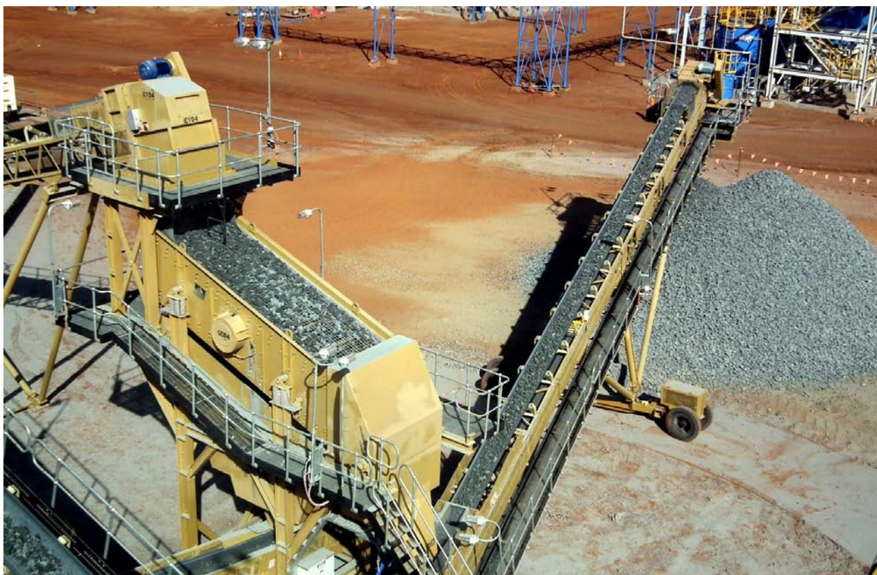
Figure 2: Scalping screen used for removal of the coarse (+40mm) native copper
