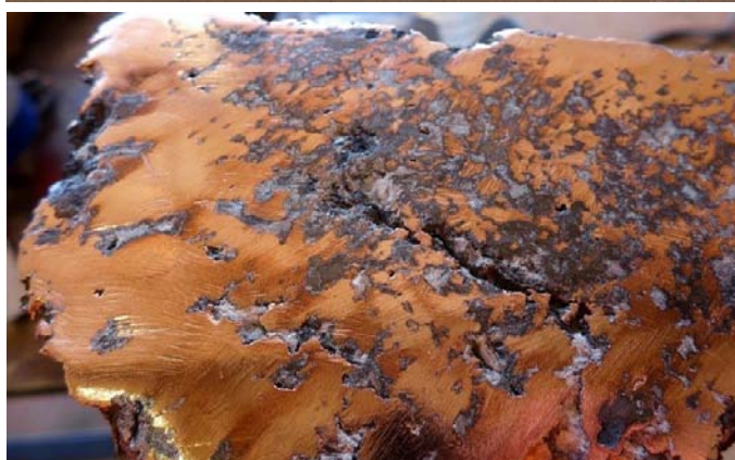
Figure 20 (above): large predominately native copper mass weighing ~130kg, with marks from the mobile jaw crusher imprinted onto its surface. This sample did not appear particularly solid at first glance (see Figure 18 previous page), but once a thin layer of surface rock was removed with a hammer, near solid copper metal was revealed.
