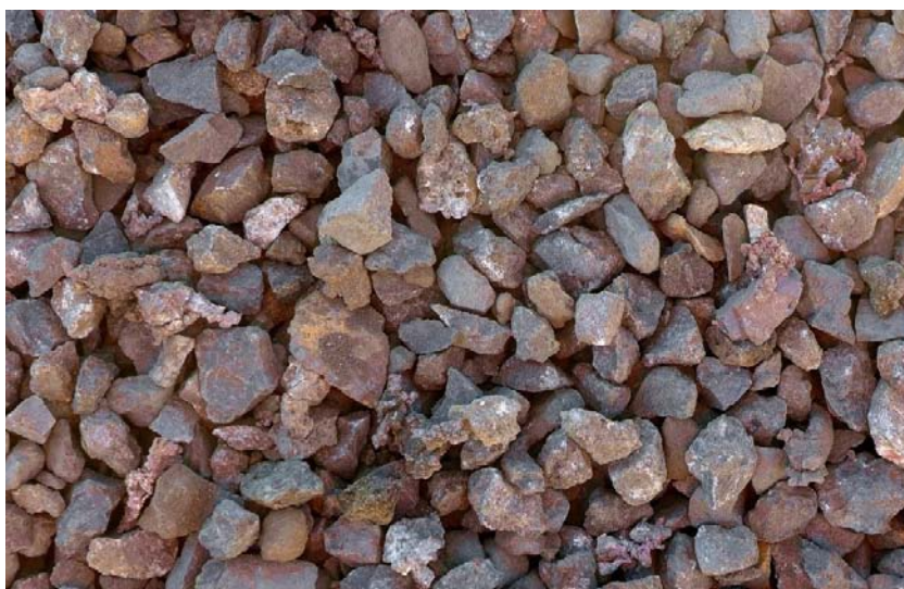
Figure 13: Close up of above crushed (-40mm) native copper ore stockpiles - ready for upgrading to a premium grade concentrate through the Company's new ore sorter to be supplied from Hamburg Germany. The above image shows coarse native copper nuggets, coarse and fine native copper in rock matrix, chalcocite, cuprite and various secondary copper species, visually estimated at 26% Cu in the above image.
