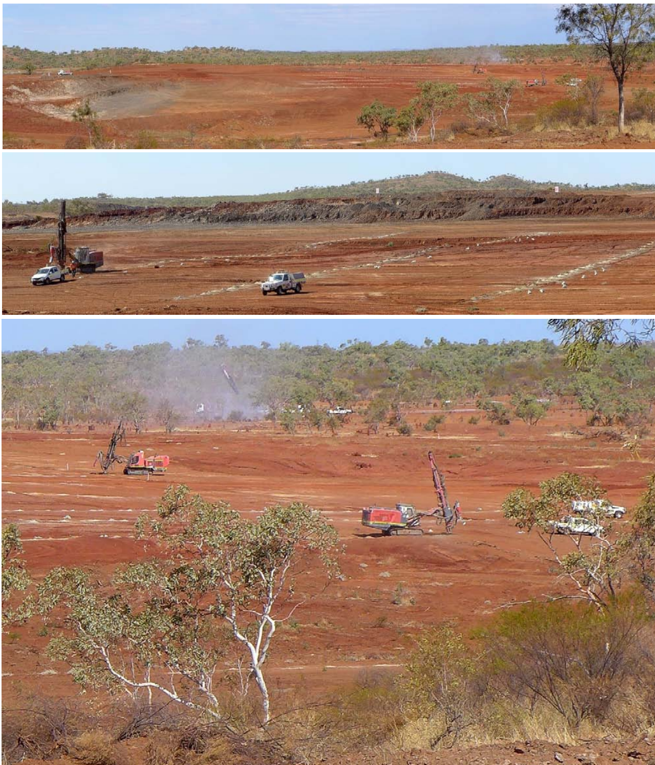
Figure 51: CuDeco is undertaking shallow bedrock drilling to help define ore zones in free-dig areas where there will be no blast-hole drilling for sampling and analysis. The Rocklands Resource model has conservatively excluded shallow ore to an arbitrary upper cut-off level which is well below the upper colluvium profile, however shallow drilling is defining wide zones of additional ore. In the top image, the initial cut-back (seen to the left) represents less than 10% of the total RS2 Pit area, but has already generated an additional 50kt of ore literally from surface, not previously included in the mining model. In the far distance is an RC rig drilling along strike from the CuDeco ore zones, as projected into the neighbouring EPM. This RC drilling is not being undertaken by CuDeco.
