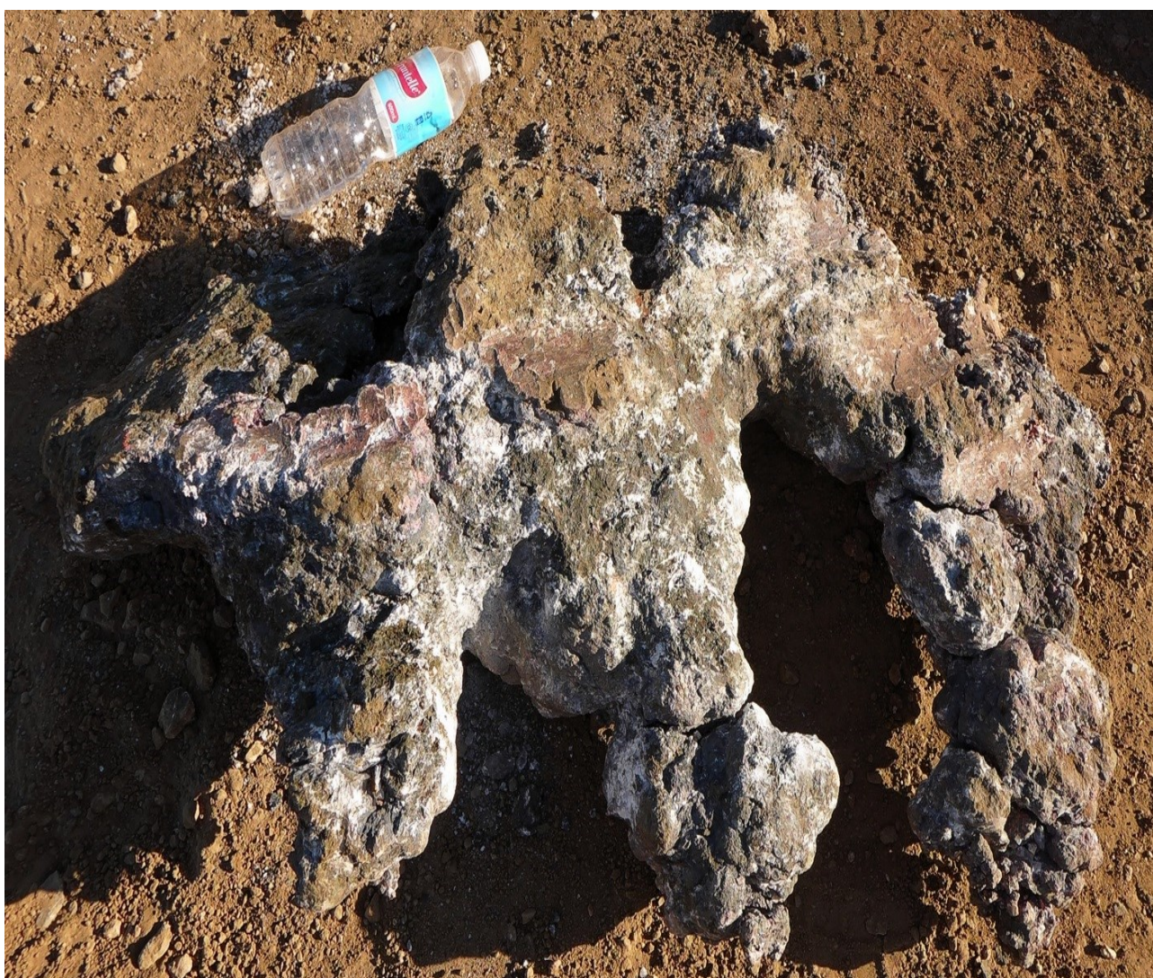
Figure 19: Large 130kg predominately native copper mass, with marks from the jaw crusher imprinted onto its surface. See following page for further details.
