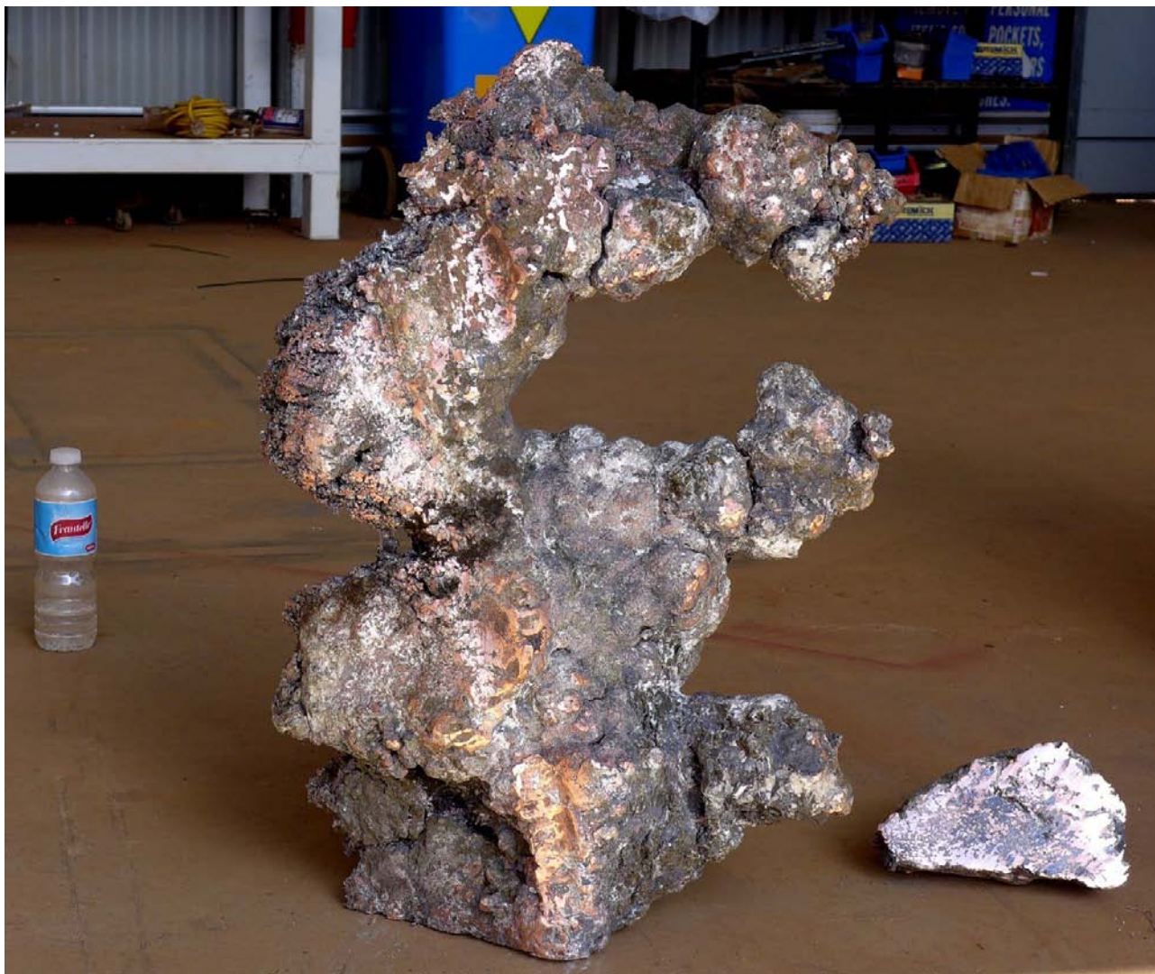
Figure 20 (above): large predominately native copper mass weighing ~130kg, with marks from the mobile jaw crusher imprinted onto its surface. This sample did not appear particularly solid at first glance (see Figure 18 previous page), but once a thin layer of surface rock was removed with a hammer, near solid copper metal was revealed.
