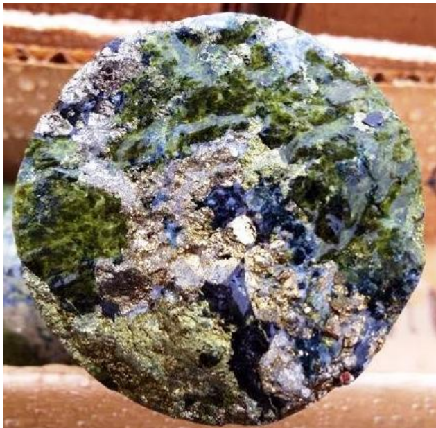
Figure 2: Photo of DDH P2-001 at 110.85m: Garnet skarn with strong epidotic retrograde magnetite / chalcopyrite / pyrite.
