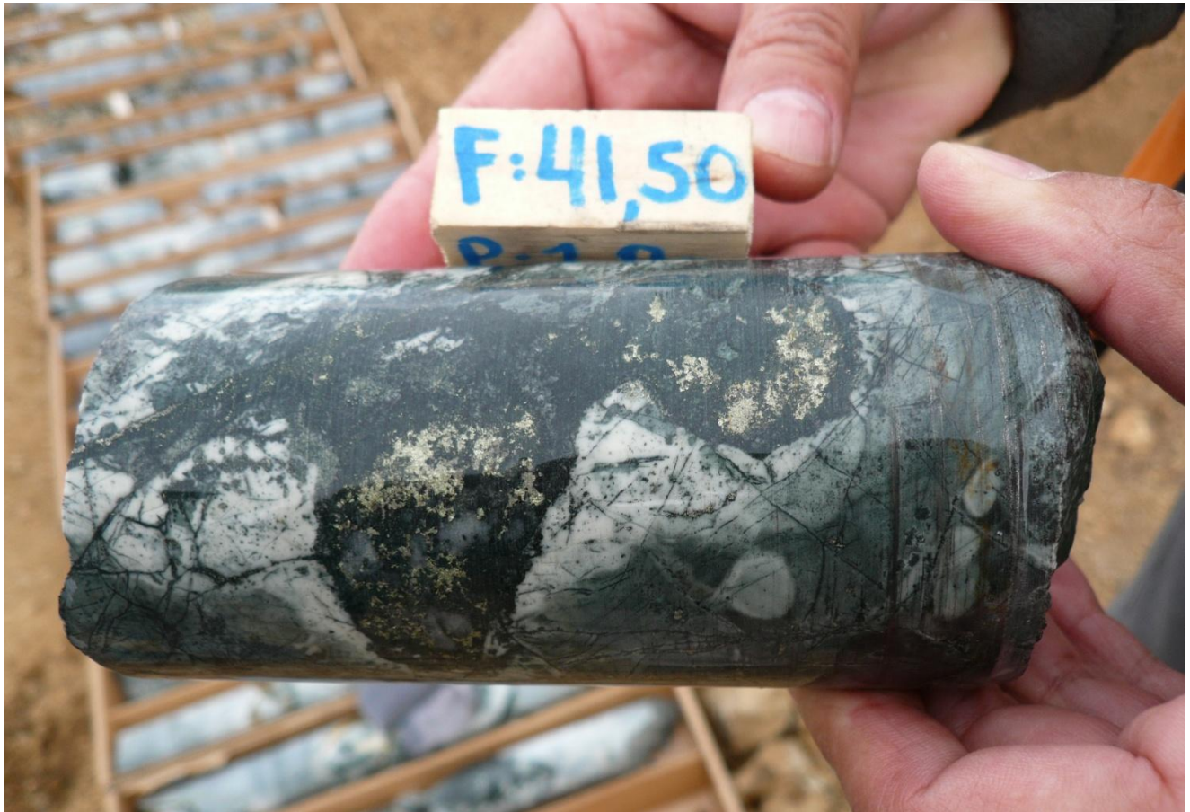
Figure 3: Photo of DDH P2-003 (Polvareda 2) at 41.5m: Clear indications of mineralisation in drill hole 1 of the re-commenced program.
