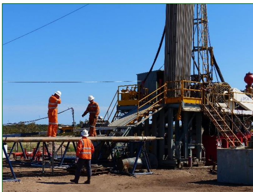
Crocker Group personnel with Key's Wellsite Geologist rigging up for wireline logging.
